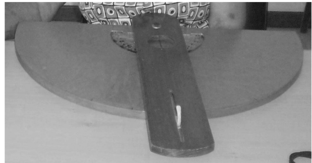
Figure 1 – Kinesimeter: instrument to evaluate the proprioception of upper limbs, according to the Paixão's Protocol (photo taken by the researchers)
