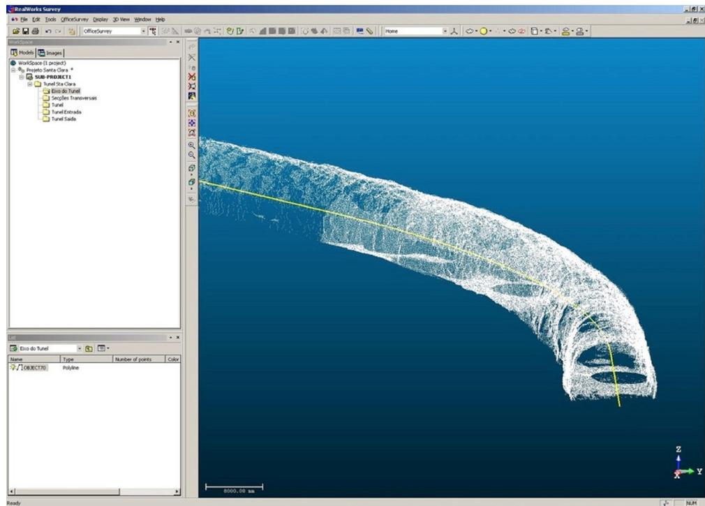
Figure 5 – General point cloud of a pipeline and its axis.
