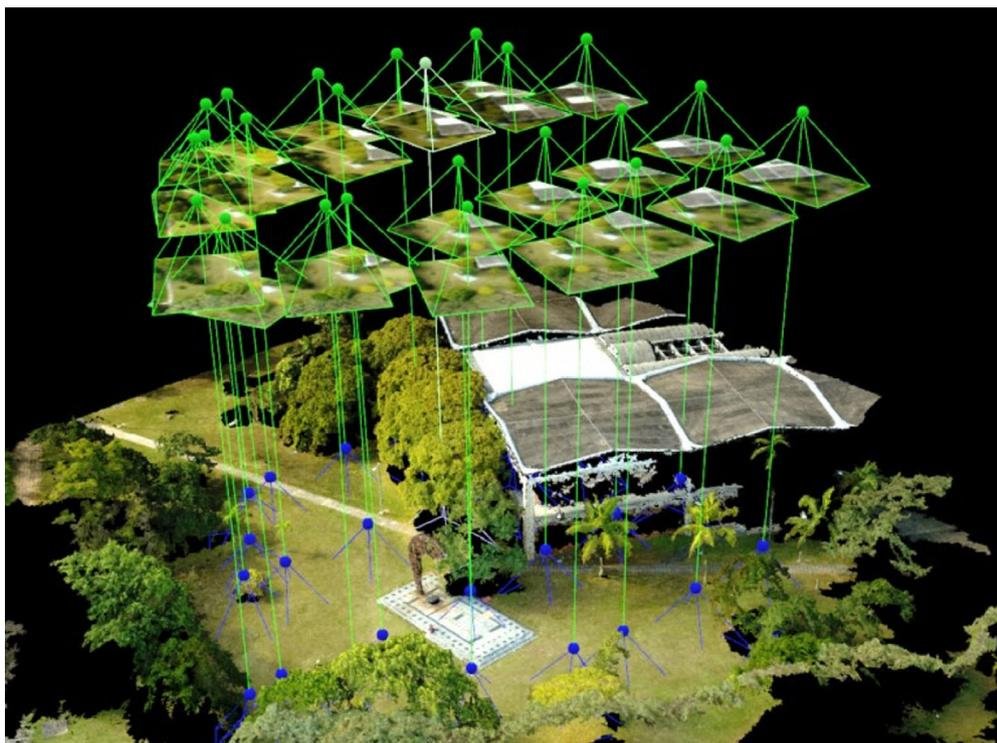
Figure 14 – Model obtained using drone, showing the flight plan.
