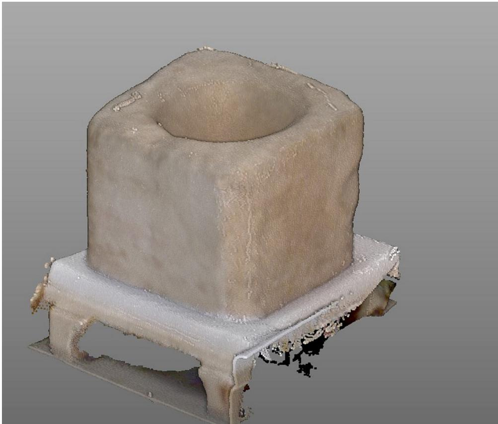
Figure 10 – Cropped point cloud showing only the mortar. Photograph by the authors.
