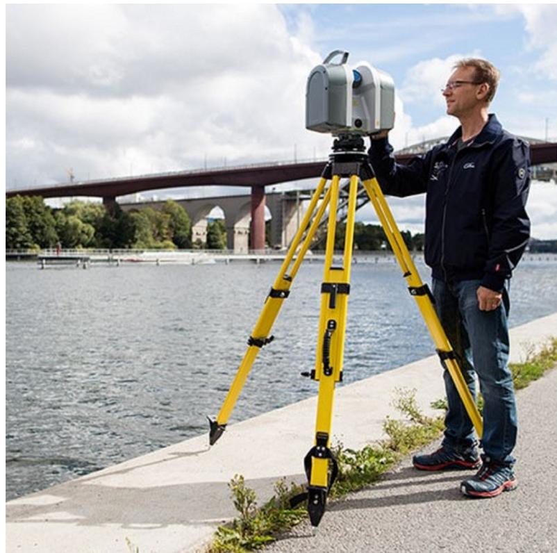
Figure 2 – Trimble TX8 3DLS, which was used to carry out several experiments for this study.
