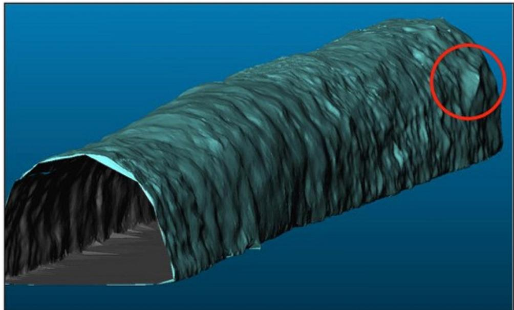
Figure 11 – 3D model of a water pipeline allowing analysis and quantifications.
