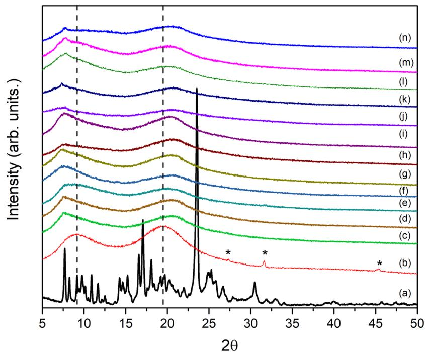
**FIGURE 2** - X-ray powder diffraction patterns of DOX (a), HPMC E6 (b), WP-F1 (c), WP-F4 (d), WP-F7 (e), F1 (f), F2 (g), F3 (h), F4 (i), F5 (j), F6 (k), F7 (l), F8 (m), and F9 (n).
