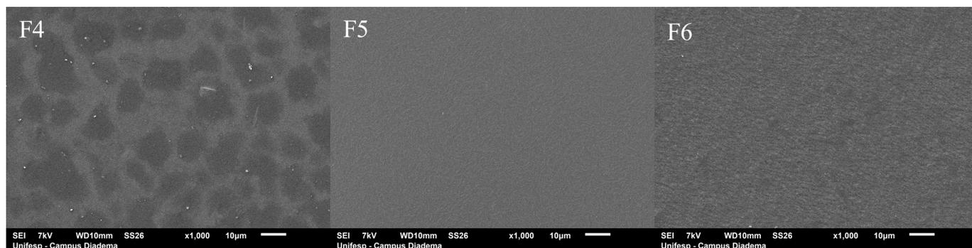
**FIGURE 5** - Photomicrographs of orodispersible films obtained using scanning electron microscopy (SEM) Jeol with an increase of 1,000x.
