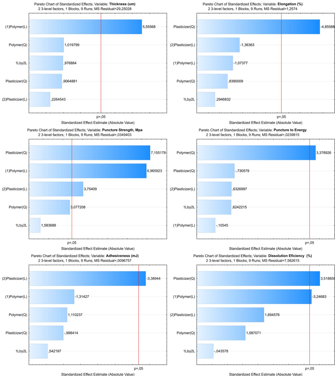
**FIGURE 3** - Pareto chart of the main effects of variables (polymers and plasticizers) on the investigated responses
