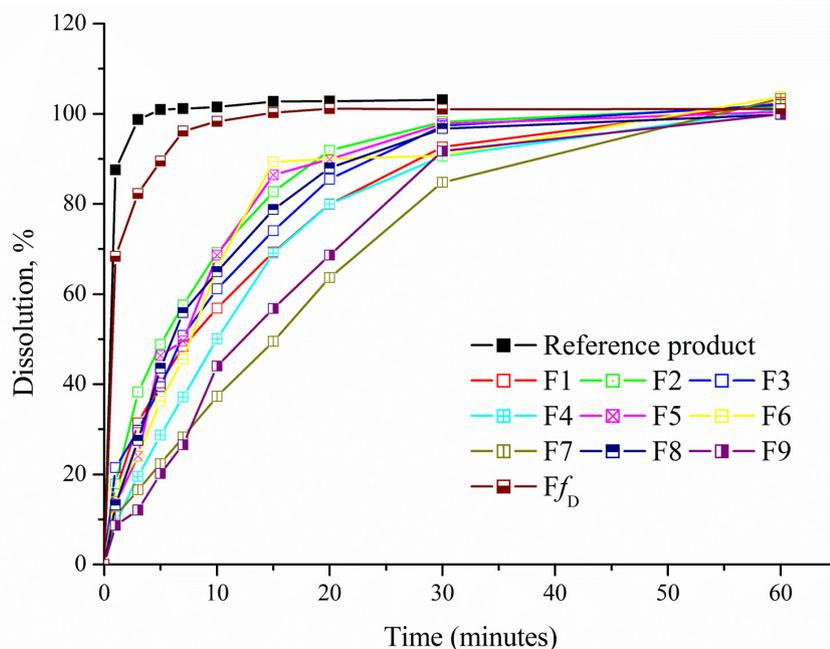
**FIGURE 6** - Dissolution profiles of orodispersible films (F1-9) and the reference product (Cardura™ 2 mg tablets; Pfizer Inc., Brazil).
