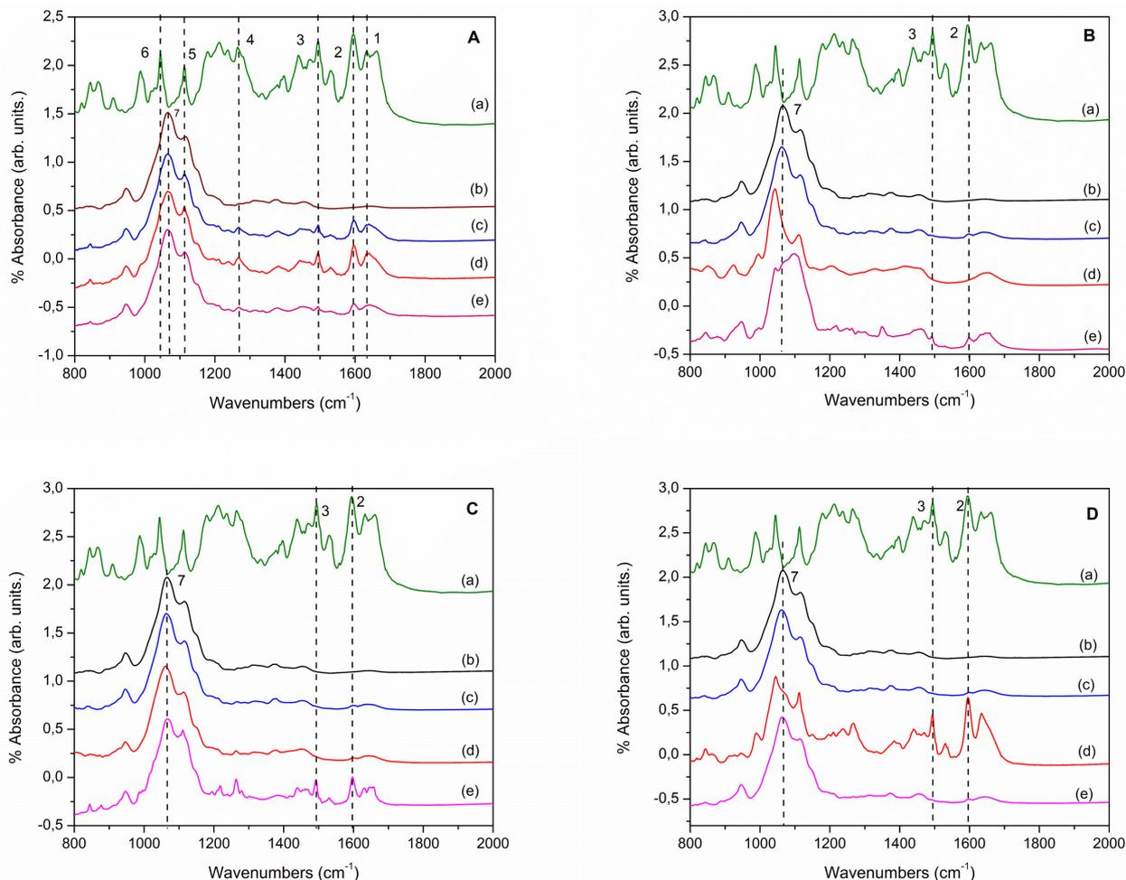
**FIGURE 1** - Fourier transformed infrared (FTIR) spectra of panel (A): doxazosin mesylate (DOX) (a), hydroxypropyl methylcellulose (HPMC) E6 (b), without plasticizer (WP)-F1 (c), WP-F4 (d), and WP-F7 (e); panel (B): DOX (a), HPMC E6 (b), F2 (c), F1 (d), and F3 (e); panel (C): DOX (a), HPMC E6 (b), F5 (c), F4 (d), and F6 (e); and panel (D): DOX (a), HPMC E6 (b), F8 (c), F7 (d), and F9 (e).
