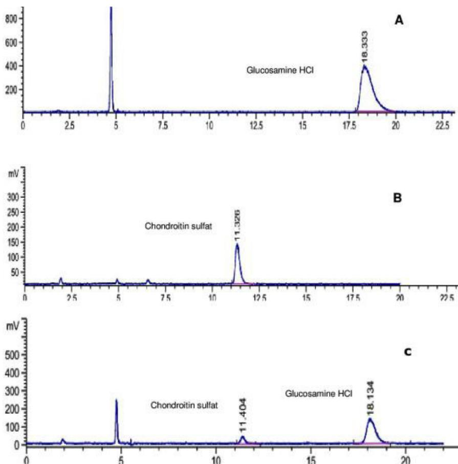
**FIGURE 2**- Chromatogram of (A) standard of glucosamine hydrochloride; (B) standard of chondroitin sulfate; (C) standard mixture of glucosamine hydrochloride and chondroitin sulfate using a HILIC-HPLCELSD with mobile phase of acetonitrile:water:30 mM ammonium format (77:3:20, v/v/v), pH 4.5, ELS detector, injection volume  $5 \mu\text{L}$ .
