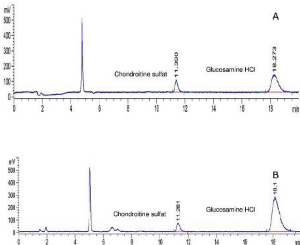
**FIGURE 3** - Chromatogram of (A) matrix spiked of standard glucosamine hydrochloride and chondroitin sulfate, (B) sample using a HILIC-HPLC-ELSD with mobile phase of acetonitrile:water:30 mM ammonium format (77:3:20, v/v/v), pH 4.5, ELS Detector, injection volume 5  $\mu$ L.
