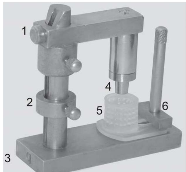
**FIGURE 1-** Apparatus used to take the impressions: 1) the upper part slides on the vertical axis of the base until it reaches a stop (2); 3) base of the apparatus; 4) steel die; 5) perforated acrylic impression tray fixed at the base of the apparatus with a metallic screw and bar (6)
